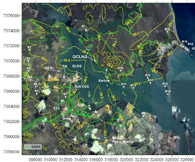
Figure 24 Scenario 1 - Predicted maximum 24-hour average ground-level concentrations of PM 10 for the QCLNG plant during normal operations, with background
