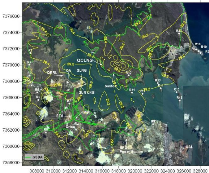
Figure 24 Scenario 1 - Predicted maximum 24-hour average ground-level concentrations of PM<sub>10</sub> for the QCLNG plant during normal operations, with background
